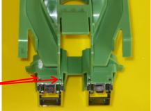
5. Install the cover and the dummy plug into the non used cable entry.
