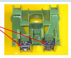
4.Remove the dust cap from the xs500 module.
