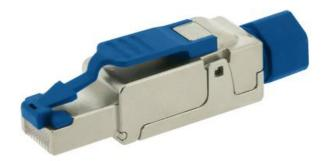
The GIGAMEDIA field plug offers the advantage of a fast and easy assembly in the field - without specific tool. The solid zinc die cast housing ensures best EMC-characteristics especially in the industrial setting. The insulation displacement and a low contact resistance guarantee the safest bonding of the cable up to 8 mm thick connection cables with the cross sections AWG23/1 - AWG26/1
