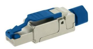
The GIGAMEDIA field plug offers the advantage of a fast and easy assembly in the field - without specific tool. The solid zinc die cast housing ensures best EMC-characteristics especially in the industrial setting. The insulation displacement and a low contact resistance guarantee the safest bonding of the cable up to 8 mm thick connection cables with the cross sections AWG23/1 - AWG26/1
