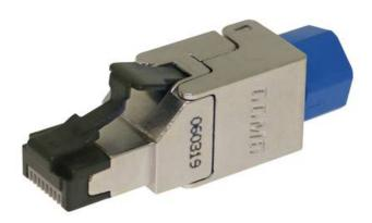
The GIGAMEDIA field plug offers the advantage of a fast and easy assembly in the field - without specific tool. The solid zinc die cast housing ensures best EMC-characteristics especially in the industrial setting. The insulation displacement and a low contact resistance guarantee the safest bonding of the cable up to 8 mm thick connection cables with the cross sections AWG23/1 - AWG26/1
