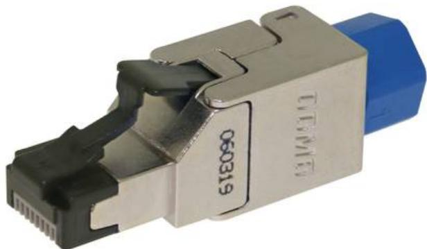
The GIGAMEDIA field plug offers the advantage of a fast and easy assembly in the field - without specific tool. The solid zinc die cast housing ensures best EMC-characteristics especially in the industrial setting. The insulation displacement and a low contact resistance guarantee the safest bonding of the cable up to 8 mm thick connection cables with the cross sections AWG23/1 - AWG26/1
