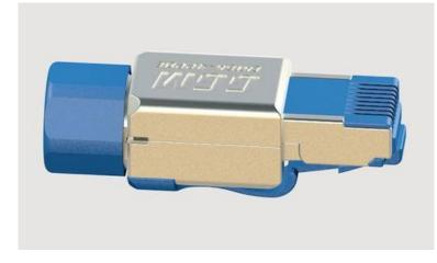
The GIGAMEDIA field plug offers the advantage of a fast and easy assembly in the field - without specific tool. The solid zinc die-cast housing ensures best EMC-characteristics. The insulation displacement and low contact resistance guarantee the safest bonding of the cable up to 8 mm thick connection cables with the cross-sections AWG23/1 - AWG26/1.
