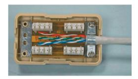
**Step 3:** Peel off the sheath of each cable about 3 cm and attach them to the cable housing one at a time.
