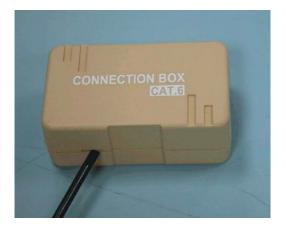
**Step 1:** Insert a screwdriver into the hole and open the housing carefully.
