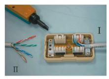
**Step 4:** Insert the cable wires in the correct positions according to the color codes (T568B).
