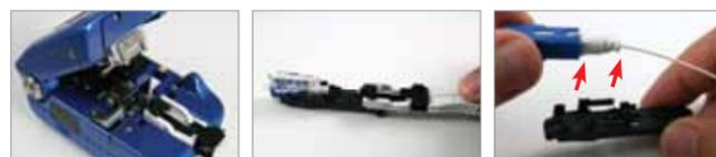
▶ 1 Cutting Fiber   ▶ 2 Inserting Fiber   ▶ 3 Take Out Connector
