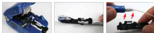
▶ 1 Cutting Fiber   ▶ 2 Inserting Fiber   ▶ 3 Take Out Connector
