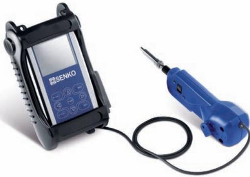
The FTTX FIBERVIEW ultra light analogue probe connects to the extremely rugged and compact 2.5" TFT hand-held monitor with a display magnification of x150 (x200 option available on request). The analogue probe is side mounted on the monitor. An additional optional probe allows the user to inspect both patchcord and In-adapter end face in one process.
