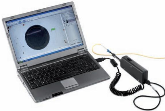
The Digital FIBERVIEW probe receives all of its power supply requirements through direct connection to the USB port on either a PC or Laptop. The probe supports variable magnification which is controlled via a proprietary software suite. This software suite also permits the end user to complete a full, automatic analysis of the ferrule end face, as viewed, for contamination and scratches against user-definable accept/reject criteria.
