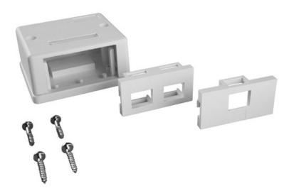
This modular surface-mount box is dedicated to allow the installation of two keystone type modules. It has been designed to make the module replacement easier. This solution allows for quick network modernization without the need to replace the entire box. The box can be mounted on the wall with screws or double-sided self-adhesive foam.
