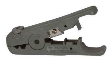
Fast and easy outer jacket removal, from all unshielded/Shielded twisted pair. GGM 907X501 offer a self-adjusting blade to stick to all different outer jacket diameter cable without damaging the inner braids, foils or conductors.
