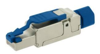
The GIGAMEDIA field plug offers the advantage of a fast and easy assembly in the field - without specific tool. The solid zinc die cast housing ensures best EMC-characteristics. The insulation displacement and a low contact resistance guarantee the safest bonding of the cable up to 8 mm thick connection cables with the cross sections AWG23/1 - AWG26/1
