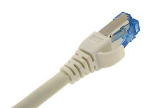
All Cat.6A screened patch cords incorporate short body blue plugs (50?) that use an integral pair manager to optimize performance and reducing untwisting of conductors within the plug, Slim Snagless molded boots are incorporated which increase protection of the plug latch, offer maximum strength construction.
