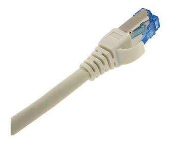
All Cat.6A screened patch cords incorporate short body blue plugs (50?) that use an integral pair manager to optimize performance and reducing untwisting of conductors within the plug, Slim Snagless molded boots are incorporated which increase protection of the plug latch, offer maximum strength construction.
