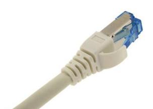
All Cat.6A screened patch cords incorporate short body blue plugs (50?) that use an integral pair manager to optimize performance and reducing untwisting of conductors within the plug, Slim Snagless molded boots are incorporated which increase protection of the plug latch, offer maximum strength construction.
