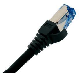
All Cat.6A screened patch cords incorporate short body blue plugs (50?) that use an integral pair manager to optimize performance and reducing untwisting of conductors within the plug, Slim Snagless molded boots are incorporated which increase protection of the plug latch, offer maximum strength construction.
