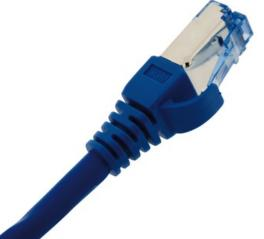
All <u>Cat.6A</u> soreened patch cords incorporate short body blue plugs (50?) that use an integral pair manager to optimize performance and reducing untwisting of conductors within the plug, Slim Snagless molded boots are incorporated which increase protection of the plug latch, offer maximum strength construction.
