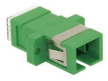
Fibre optic adapters (or bulkheads) are used to connect two connectors ferrules (eg pigtails, patchcords) together and ensure signal continuity. The central sleeve of the adapter guarantees perfect mechanical mating to optimize insertion loss & reflectance.
