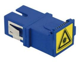
Adapters (or bulkheads) ar used to connect two fibers (loaded with connectors i.e pigtails, patchcords, ...) together. The central sleeve of adapters ensures fiber connectors are perfectly mated together to optimize Insertion Loss & reflectance.
