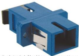
Fibre optic adapters (or bulkheads) are used to connect two connectors ferrules (eg pigtails, patchcords) together and ensure signal continuity. The central sleeve of the adapter guarantees perfect mechanical mating to optimize insertion loss & reflectance.
