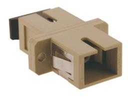
Adapters (or bulkheads) ar used to connect two fibers (loaded with connectors i.e pigtails, patchcords, ...) together. The central sleeve of adapters ensures fiber connectors are perfectly mated together to optimize Insertion Loss & reflectance.
