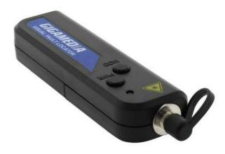
With its 1 mW output power, the VFL1MW allows testing signal continuity and detecting possible breaks on a fibre optic link up to 5 km.
