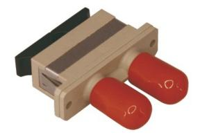
Adapters (or bulkheads) ar used to connect two fibers (loaded with connectors i.e pigtails, patchcords, ...) together. The central sleeve of adapters ensures fiber connectors are perfectly mated together to optimize Insertion Loss & reflectance.
