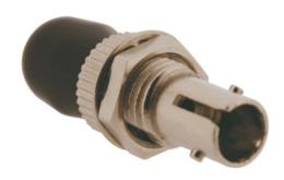
Adapters (or bulkheads) ar used to connect two fibers (loaded with connectors i.e pigtails, patchcords, ...) together. The central sleeve of adapters ensures fiber connectors are perfectly mated together to optimize Insertion Loss & reflectance.
