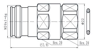
4.3-10 Straight female Connector for 1/2" Flexible RF Cable
