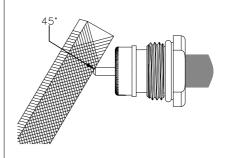
9 The cable center conductor must be straight and aligned with the connector inner contact. Insert the cable into the connector body until stopped; the center conductor must be inserted into the connector inner contact holes.
