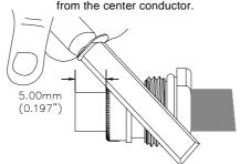
8 Chamfer the center conductor at a 45° angle. It is very important.
