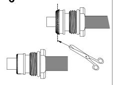
Removed 5.0 mm (0.197") foam. Removed all foam/glue residue from the center conductor.
