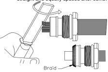
Cut off the redundant braid as shown.
