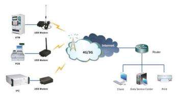
RTU (Remote Terminal Unit) is a cellular communication device installed at a remote location that collect data, codes the data into a format that is transmittable and transmit the data back to a central station or master, it is been developed especially for data collection and data transmission in IoT / M2M application.
