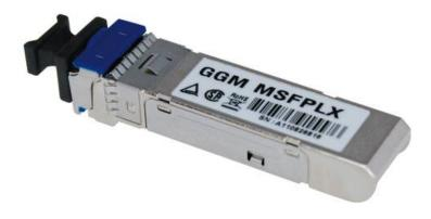
The GIGAMEDIA small form-factor pluggable (SFP) or Mini-GBIC is a hot-pluggable transceiver, compact used for data communications applications, supporting full duplex for Fast or Gigabit Ethernet speeds on multimode fiber or singlemode fiber for long distances. These modules are in "LC" connector, they interfaces a network device mother board (into a switch, media converter etc) to a fiber optic networking cable. This format is supported by many network component vendors.
