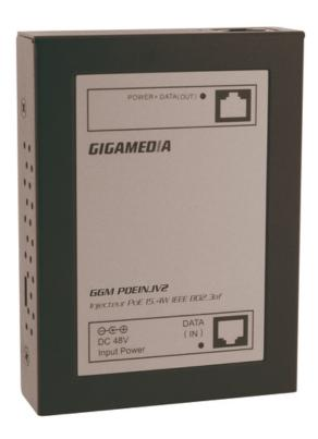
GGM POEINJV2 is 1 Ethernet Input (data only) port and 1 Output (data + power) port Power over Ethernet Injector that is designed for small or medium network environment to strengthen its network connection. This product can convert standard 12~24V/DC or 48V/DC power into DC voltage that runs over existing LAN cable to power up IEEE 802.3af compliant network accessory
