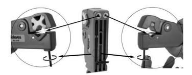
Cut and outer sheath removal
