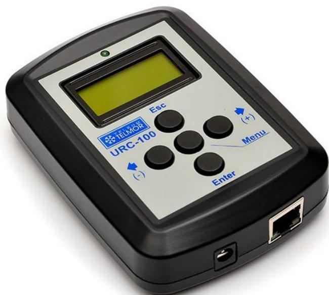
The **URC-100 controller/ programmer** is an external manipulator which enables correct programming of **WWK-9NG, WWK-IQ USB, SWK-9216** devices. Access to the whole menu of these devices is possible only with the controller.
