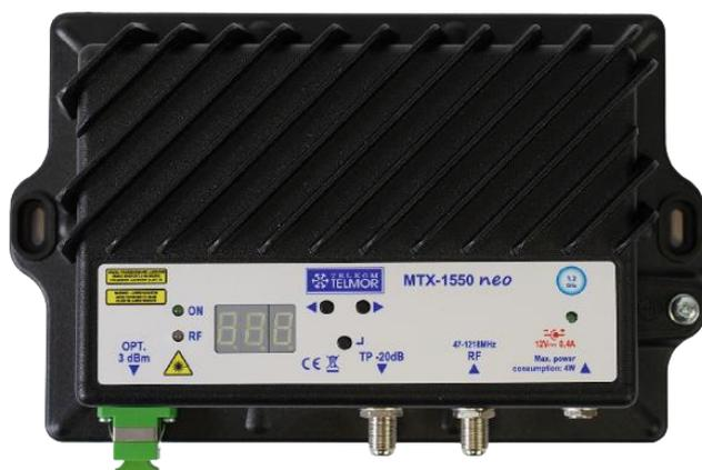
MTX neo is an optical transmitter with a optical output power of 0, 3 or 6 dBm. It enables input of an RF signal in the frequency range of 47-1218 MHz. The signal from the transmitter through the SC / APC connector is distributed over one optical fiber. The connected signal should be automatically adjusted thanks to AGC technology. The MTX neo optical transmitter allows you to send a signal at a distance of up to 20 km.
