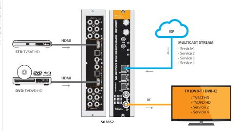
The Encoder / Modulator generates a RF Mux with services transmitted through IP Multicast, supplied by an operator and with A/V signals.
