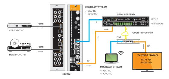
The Encoder / Modulator generates a RF Mux and a Multicast stream with A/V signals.
