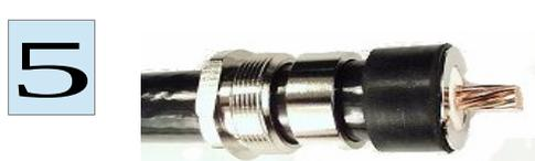
Remove the copper foil and the dielectric with a knife. The inner conductor must stay absolutely round. Remove burr from sharp edges.
