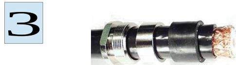
Remove 10 mm of the outer sheath with a knife.
