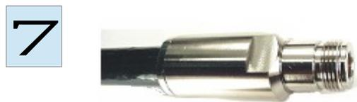
The prepared cable tail has to be inserted into the housing until stop. Tighten the clamping nut finger tight with two open-ended spanners 19 mm. A small split should remain visible between clamping nut and connector housing.
