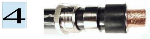
Bend copper braid upwards right-angled. Heat the cable with the hot air gun. (abt. 150°C) Insert contact sleeve between copper foil and braid until stop. Cut off protruding braid. Move the rubber seal to the front, up to the contact sleeve.
