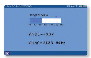
The measurement of the DC and AC voltages present at the RF input is displayed together with the total RF power for convenience.
