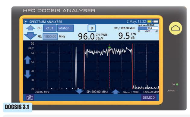
DOCSIS 3.1 systems can use among other things an extended frequency range which goes up to 1500 MHz in the forward path with a return band up to 200 MHz. The **CABLE RANGER** RF input covers up to 1700 MHz.
