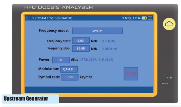
A frequency and amplitude agile return path generator is also available in the **CABLE RANGER**. It allows generating a test signal which can be tuned from 5 to 85 MHz and it can be CW or modulated in QAM and QPSK. It can also be configured to sweep a specific frequency range within that band.
