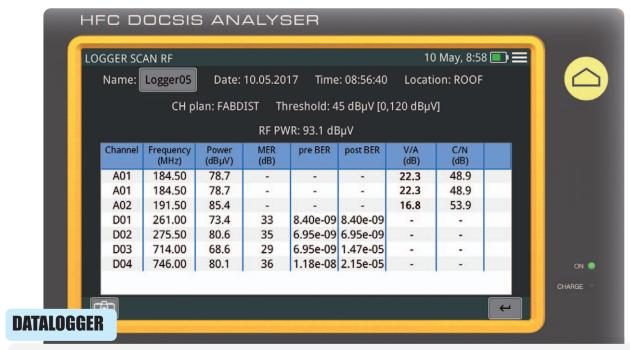
The datalogger function can perform various measurements including signal level and channel power, carrier/noise, BER and MER for all the channels listed in a given channel table automatically. All this information is saved in the analyzer and it can be copied to a pendrive or to a PC for further processing at a later stage.
