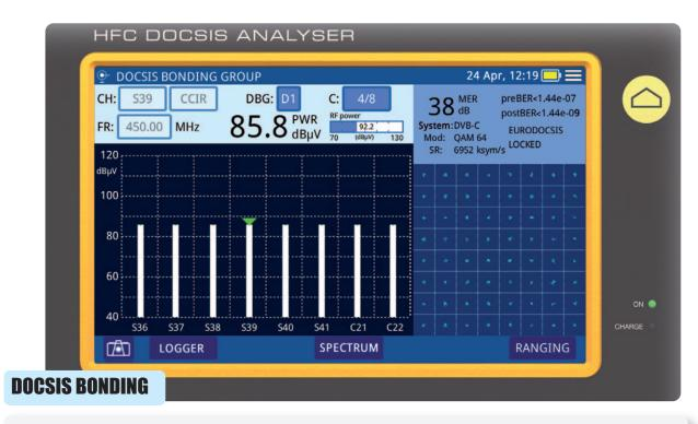
As part of the DOCSIS 3.0 standard multiple upstream and downstream channels can be 'bonded' to be used together as one. **CABLE RANGER** includes a comprehensive channel bonding screen where information about all of them is combined with other single channel measurements such as the constellation diagram.
