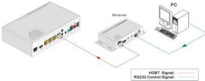
**Figure 4- 4 Control local device from remote**
