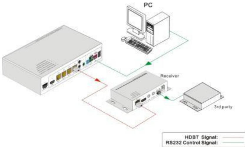
**Figure 4- 3 Control far-end device from local**
