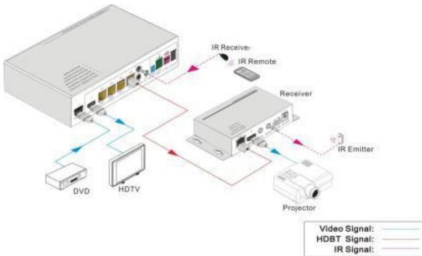
**Figure 4- 1 Control far-end device from local**
