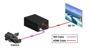
Note: RG59 cable is required for SDI transmission, we recommend a 75-ohm high quality coaxial cable.
