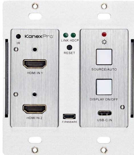
The **KanexPro WP-2XHDUSBC** is a US Decora style double-gang, 3x1 Wall plate transmitter and switcher designed to switch two HDMI®2.0 inputs and one USB-C input to a remote display or a projector up to 131ft.(40m) at 4K/60 and 230ft. (70m) at 1080p/60 video and audio over single cat5e/6/7 cable. The outputs are via HDBaseT port. It supports full 18 Gbps bandwidth with true 4K video resolutions up to 4/60Hz, HDCP 2.2 compliant and will extend 4K up to 40m delivering color sampling rate of 4:4:4.
