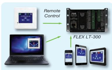
FLEX-LT300 – The LT300 is another specialty member of the Flex Family. The LT300 is basically an LT-200 in a box without a touchscreen. The LT300 can be mounted in a rack or Ceiling Box and connected to all of the devices that need to be controlled. The user interface to the LT300 is provided either by a FLEX-LT200 or LT150 or the Flex Remote Windows application.
