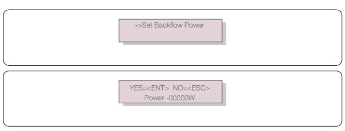
Press the UP/DOWN keys to set data. Press the ENTER key to set backflow power. Then press DOWN keys to move the cursor, press UP to change the number.
