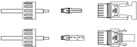
Disassemble the Connector Cap nut
