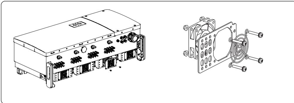
6. Disconnect the fan connector carefully and take out the fan.
