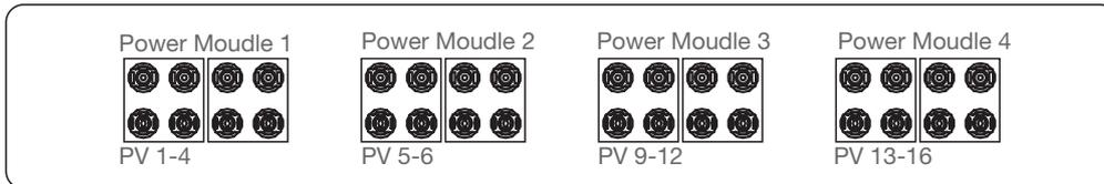
If four power modules are indeed required to connect the solar panels unevenly, for a power module which is connected to four strings, it is necessary to ensure that the power of each PV string connected under this power module does not exceed 9.2kW to achieve better power generation performance. In the case that the power difference between each PV string is less than 10% the 3 common cases are showing below.
