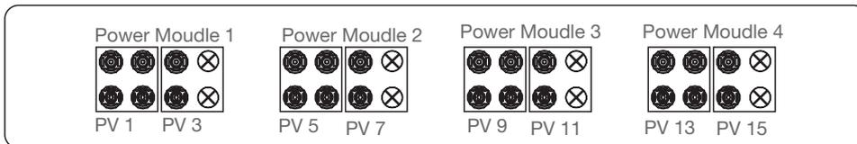
If four power modules are indeed required to connect the solar panels unevenly, for a power module which is connected to no more than three strings, it is necessary to ensure that the power of each PV string connected under this power module does not exceed 7.6kW to achieve better power generation performance. In the case that the power difference between each PV string is less than 10%, the 3 common cases are showing below.
