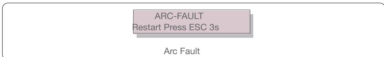
Installer needs to thoroughly inspect the DC circuit to ensure all the cables are correctly fastened. Once the DC circuit issue has been fixed or it is confirmed to be OK, press "ESC" for 3s and wait for the inverter to restart.
