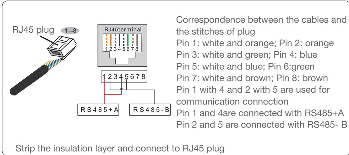
RS-485 communication through terminal board. The cross sectional area of the conductor wire for terminal board connection should be 0.2-1.5mm.
