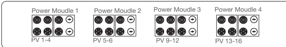
If four power modules are indeed required to connect the solar panels unevenly, for a power module which is connected to three strings, it is necessary to ensure that the power of each PV string connected under this power module does not exceed 12.2kW to achieve better power generation performance. In the case that the power difference between each PV string is less than 10%, the 3 common cases are showing below.
