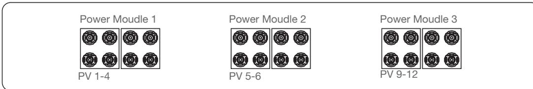
If three power modules are indeed required to connect the solar panels unevenly, for a power module which is connected to three strings, it is necessary to ensure that the power of each PV string connected under this power module does not exceed 12.2kW to achieve better power generation performance. In the case that the power difference between each PV string is less than 10%, the 2 common cases are showing below.
