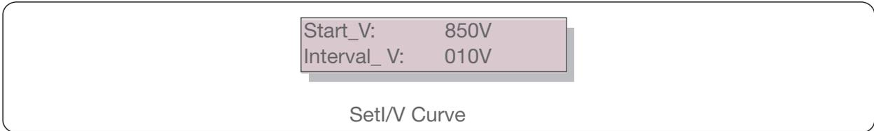
Start\_V: The start voltage of the I/V scan.(Adjustable from 300V-1000V)
