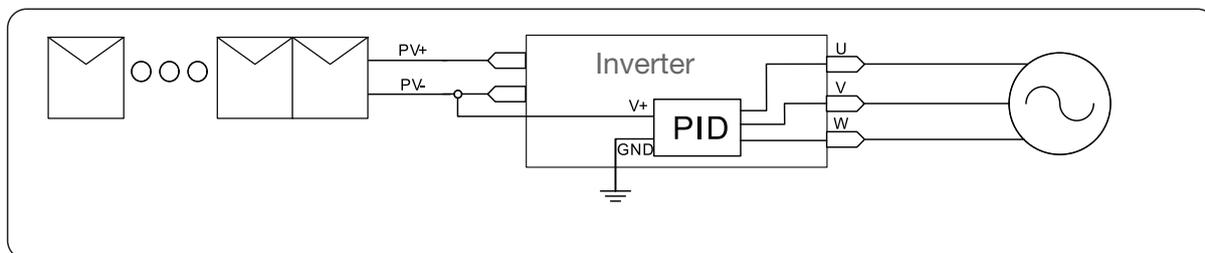
The Anti-PID module repairs the PID effect of the PV model at night. When operating, the inverter LCD screen displays "PID-repairing" information, and the red light is on. The Anti-PID function is always ON when AC is applied. If maintenance is required and turn off the AC switch can disable the Anti-PID function.
