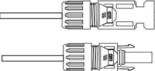
Connector with Cap nut Screwed on
