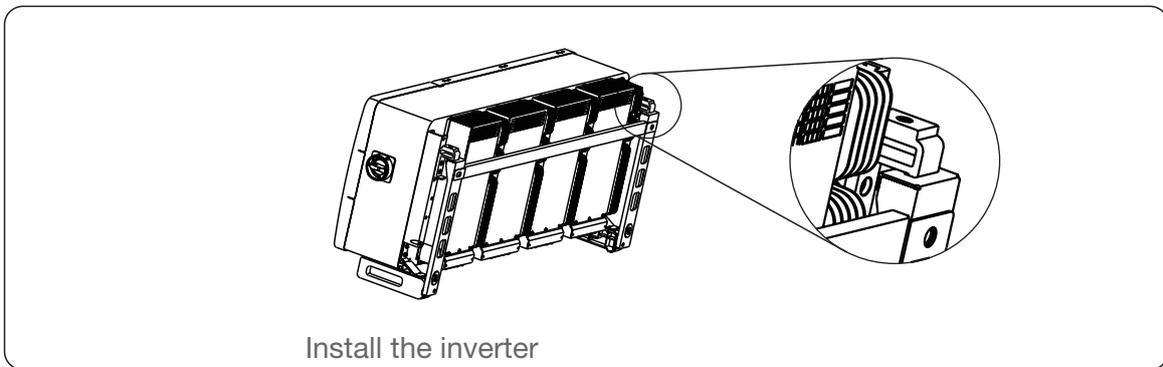
5. Use screws in the packaging to fix the inverter to the mount bracket.
