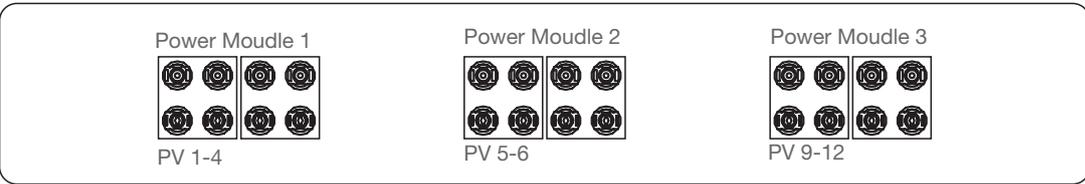
If three power modules are indeed required to connect the solar panels unevenly, for a power module which is connected to four strings, it is necessary to ensure that the power of each PV string connected under this power module does not exceed 9.2kW to achieve better power generation performance. In the case that the power difference between each PV string is less than 10% the 2 common cases are showing below.
