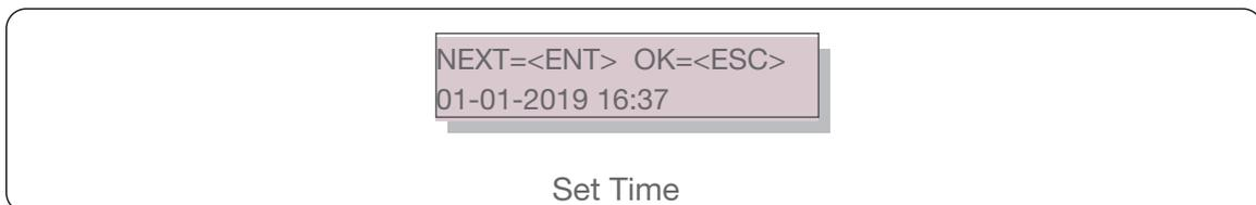
Press the UP/DOWN keys to set time and date. Press the ENTER key to move from one digit to the next (from left to right). Press the ESC key to save the settings and return to the previous menu.
