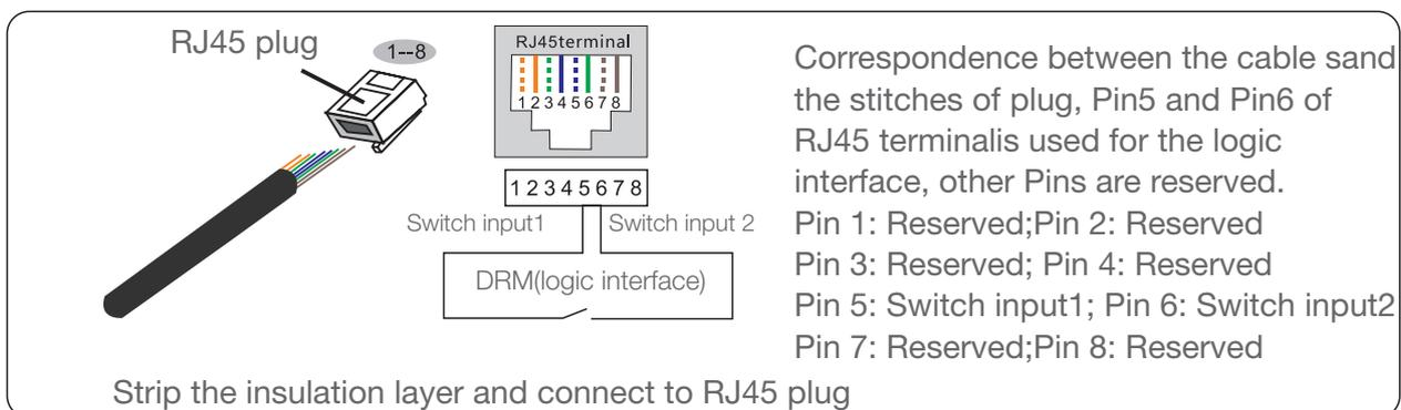
3. Connect RJ45 to DRM (logic interface)
