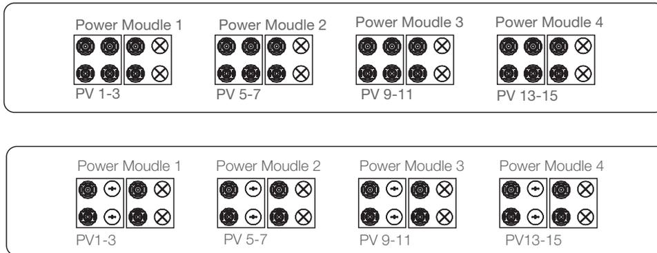
If four power modules are indeed required to connect the solar panels unevenly, for a power module which is connected to no more than three strings, it is necessary to ensure that the power of each PV string connected under this power module does not exceed 7.6kW to achieve better power generation performance. In the case that the power difference between each PV string is less than 10%, the 3 common cases are showing below.
