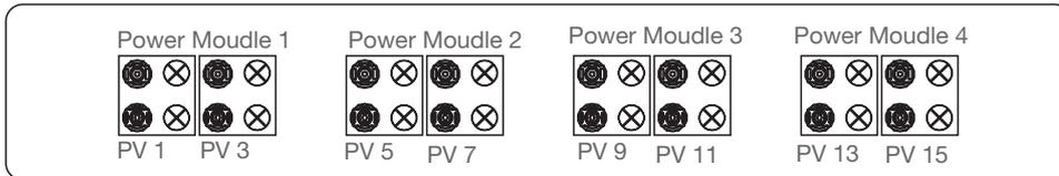
If four power modules are indeed required to connect the solar panels unevenly, for a power module which is connected to no more than two strings, it is necessary to ensure that the power of each PV string connected under this power module does not exceed 10.6kW to achieve better power generation performance. In the case that the power difference between each PV string is less than 10%, the 1 common cases are showing below.
