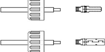
Insert the Wire into the Connector Cap nut and contact pin
