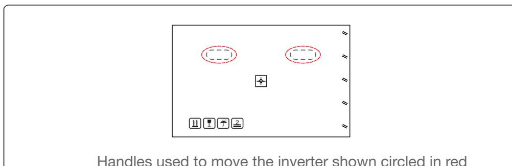
2. Two people are required to remove the inverter from the shipping box. Use the handles integrated into the heat sink to remove the inverter from the carton (see next page).
