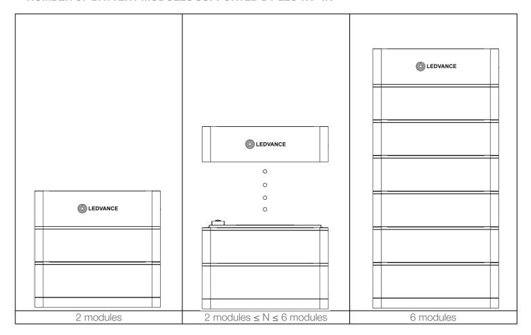
Note: Minimum two battery modules are required and Maximum Six modules in one parallel
