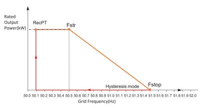
Fig. 11-3 Frq-Watt Mode for Over-frequency Conditions
