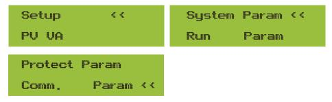
Pic 8.17 Submenus of the parameter setup
