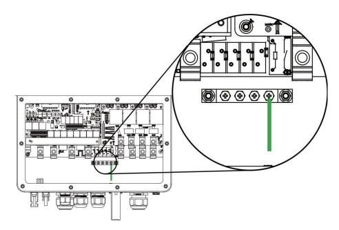
Earth connection (Copper wires)
