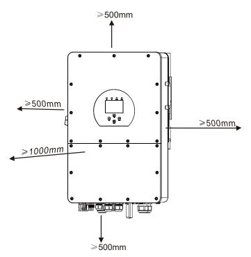
For proper air circulation to dissipate heat, allow a clearance of approx. 500mm to the side and approx. 500mm above and below the unit. And 1000mm to the front.
