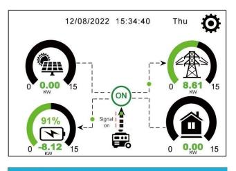
This page tells how the PV and diesel generator power the load and battery.
