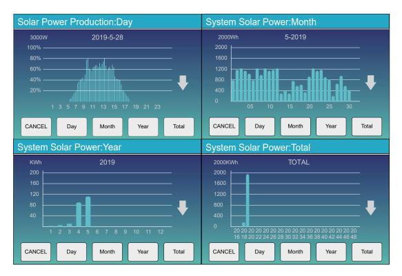
Solar power curve for daily, monthly, yearly and total can be roughly checked on the LCD, for more accuracy power generation, pls check on the monitoring system. Click the up and down arrow to check power curve of different period.
