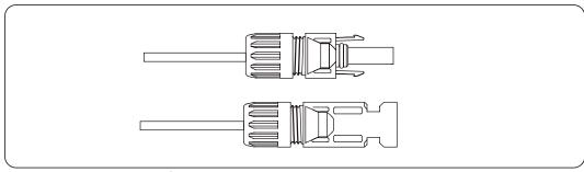
Connector with cap nut screwed on
