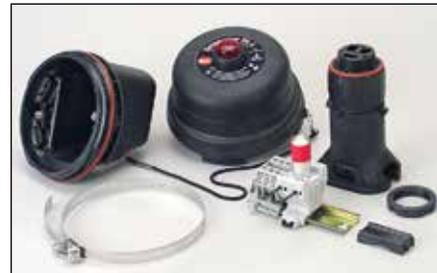
**Terminator DL** is designed to provide visual indication of an energized heating circuit. The kit may be utilized as a power connection or an end termination kit. Electrical connections are made in terminal blocks utilizing nickel-plated copper terminals to ensure corrosion-free electrical integrity.
