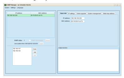
You can modify IP setting, online upgrade, password management, and static trap address setting in SNMP Manager interface. It is necessary to enter password for any medications. The default password is 12345678.
