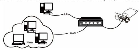
When the network interface cable is connected, the SNMP Card will attempt to obtain an IP address via DHCP. See "Configuration methods" on page 6.
