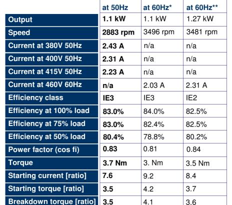
**Insulation class** F (155 °C)/ temperature rise B (80K)
