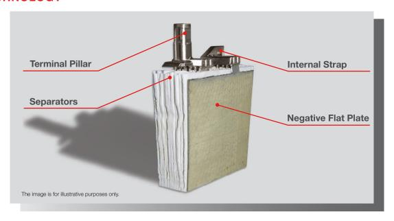
FIAMM FLB RANGE USE AGM (ABSORBED GLASS MAT) TECHNOLOGY. THE ELECTROLYTE IS ABSORBED IN FIBERGLASS SEPARATORS WITH 99% INTERNAL GAS RECOMBINATION EFFICIENCY. BLOCS ARE GRANTS NON-SPILLABLE AND MAINTENANCE FREE THEREFORE REQUIRES NO TOPPING UP OF ELECTROLYTE DURING ITS WHOLE LIFE. LOW SELF-DISCHARGE ALLOWS 6 MONTHS SHELF LIFE.
