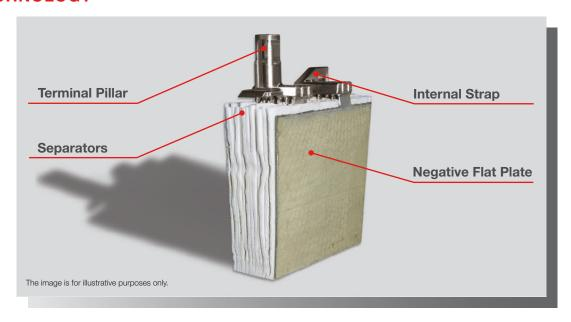
FIAMM FIT RANGE USE AGM (ABSORBED GLASS MAT) TECHNOLOGY. THE ELECTROLYTE IS ABSORBED IN FIBERGLASS SEPARATORS WITH 99% INTERNAL GAS RECOMBINATION EFFICIENCY. BLOCS ARE GRANTS NON-SPILLABLE AND MAINTENANCE FREE THEREFORE REQUIRES NO TOPPING UP OF ELECTROLYTE DURING ITS WHOLE LIFE. LOW SELF-DISCHARGE ALLOWS 6 MONTHS SHELF LIFE.
