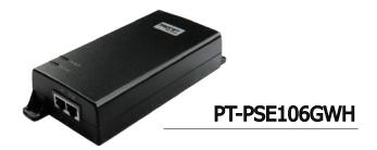
PT-PSE106GWH is designed for indoor use. It works with input voltage of 100-240 Vac. It has detection chip inside, which will detect and classify PD before powering it. It will not apply power until a standard-compliant PD is detected. The effective distance is 100 meters over Cat5e/Cat6 cables.
